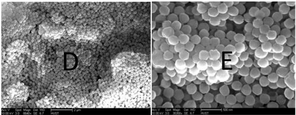
Photo FSEM ( D and E ) of Crosslinked PMMA nanoparticles
