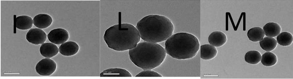
Photo ( I ,L and M ) TEM of Crosslinked PMMA nanoparticles
