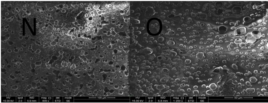
Photo ( N and O ) FSEM of Membrane of PMMA & PMMA crosslinked treated THF
