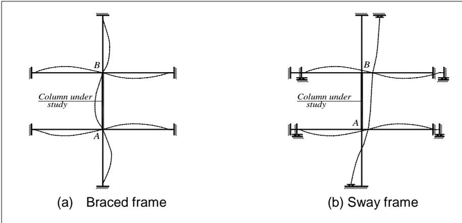
Fig. 1 Braced and sway frames
