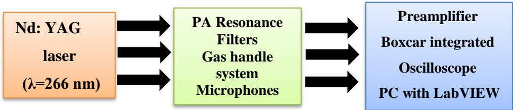
*Figure-2: Schematic layout of photoacoustic experiment.*
