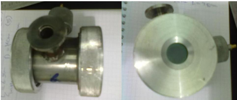
*Figure-2 : PA Cell Dimension: Length= 7.5cm & Radius =1.4cm*
